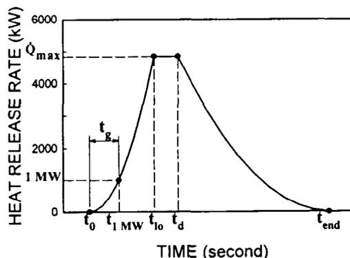
Figure 1. Heat Release Rate vs. Time in  $t^2$ -fire Characterization.
