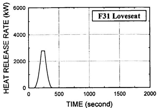
Fig. A33. F31 Loveseat, wood frame, polyurethane foam, olefin fabric
