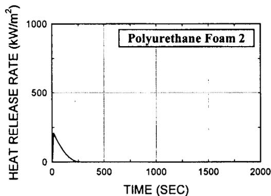
Fig. D21. Rigid polyurethane foam, gm-29/gm-30 (test 257), Foam
