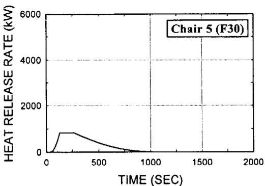
Fig. B7. Uphols.chair, F30,pu frame, pu foam, olefin, test 30 (82-2604)
