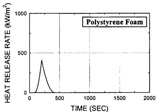
Fig. D19. Polystyrene foam, 2 in (test 437), Foam
