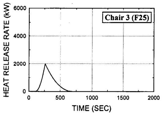
Fig. B5. Upholstered chair, F25, wood frame, pu foam, olefin, test 29
