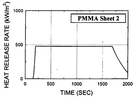
Fig. D16. PMMA 1" black (cb) w/frame (test 1470), Sheet
