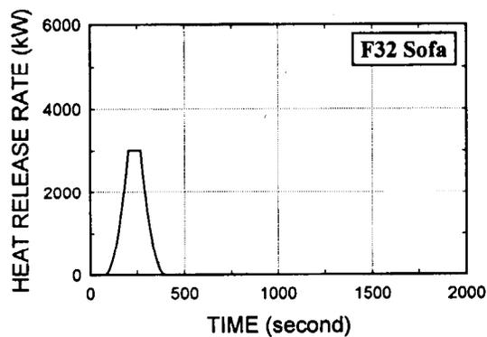
Fig. A34. F32 Sofa, wood frame, polyurethane foam, olefin fabric
