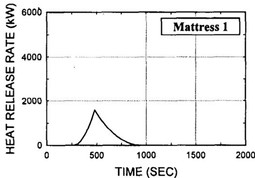
Fig. B15. Mattress, m05, pu foam, rayon ticking, bedding
