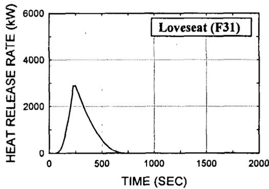
Fig. B14. Loveseat, F31, wood frame, pu foam (fr), olefin test 37 (82-2604)
