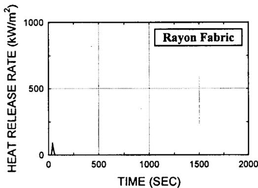
Fig. D24. Rayon fabric (test 804a), Fabric
