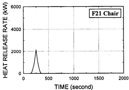
Fig. A32. F21 Chair, wood frame, polyurethane foam, olefin fabric
