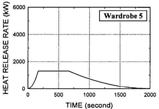
Fig. A5. 3/4" Particle-board wardrobe, thin plastic coating
