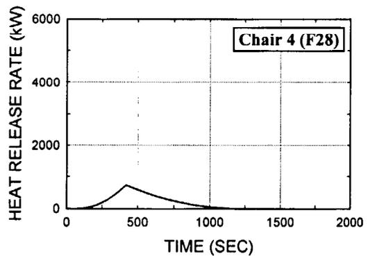
Fig. B6. Uphols.chair, F28, wood frame, pu/pe/ctn bedding, cotton test 28
