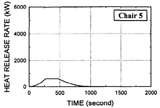
Fig. A10. Chair, wood frame, California foam, Haitian cotton fabric
