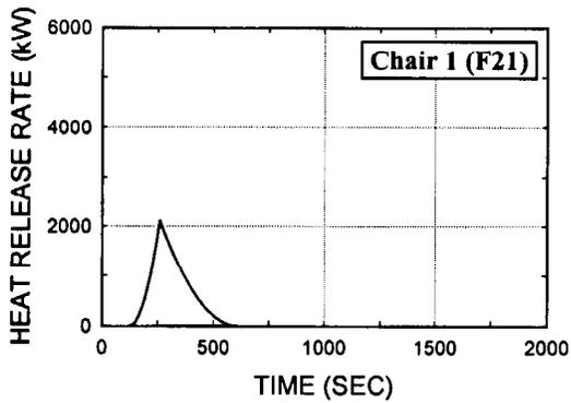
Fig. B3. Upholstered chair, F21, wood frame, pu foam-fr, olefin
