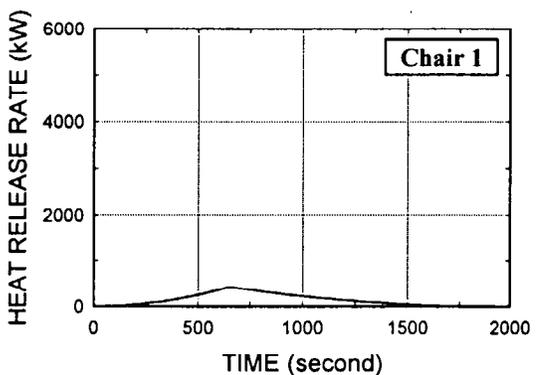
Fig. A6. Chair, one-piece wood-reinforced urethane foam
