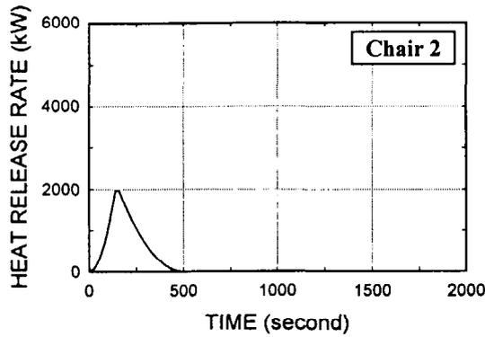
Fig. A7. Chair, polypropylene foam frame, urethane foam, polyolefin fabric
