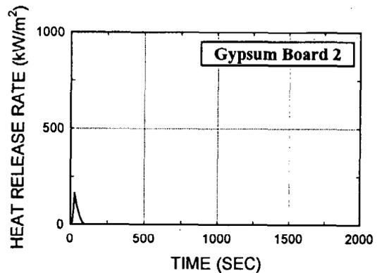
Fig. D6. Gypsum board, 1/2 in. thick (448)
