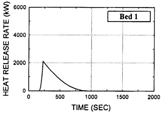
Fig. B1. Double bed, bedding, night table; gyp bd walls; test R1 (85-2998)
