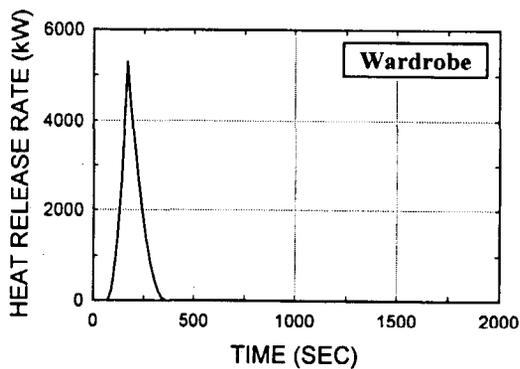
Fig. B20. Wardrobe closet, plywood, fr paint nbsir 83-2787 test 42
