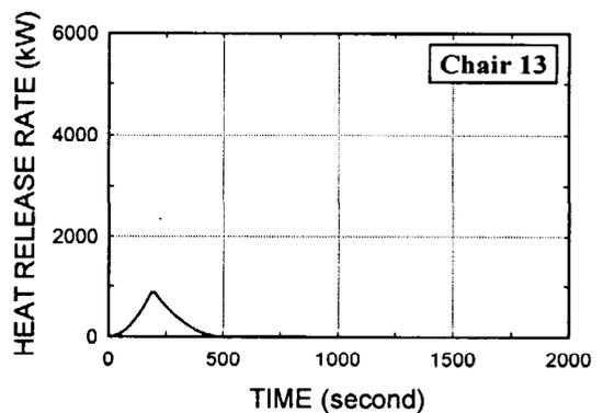
Fig. A18. Chair, wood frame, urethane foam, quilted cotton/polyolefin, polyester batting
