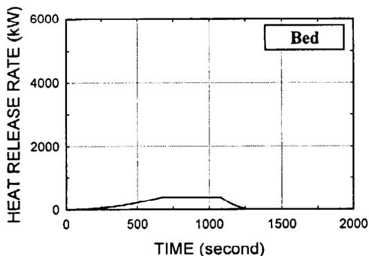
Fig. A19. Innerspring mattress and boxspring, cotton felt/urethane/sisal spring cover
