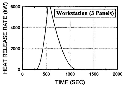
Fig. C10. Workstation (3 panels), Sponsored by GSA and performed at BFRL in 1991
