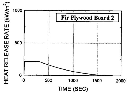
Fig. D4. Douglas fir plywood, 1/2 in. thick (446), Board
