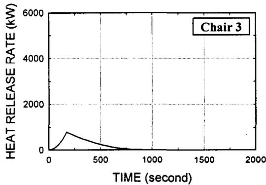
Fig. A8. Chair, thin wood frame, California foam, polyolefin fabric
