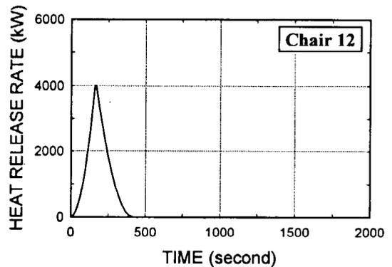
Fig. A17. Chair, wood frame, urethane foam, polyolefin fabric
