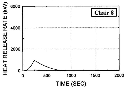
Fig. B10. Easy chair, molded ps foam frame, pu pad & cover, c07, test 48
