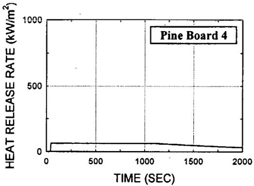
Fig. D14. White pine (wood), 0.75 in (test 493), Board
