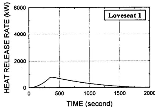
Fig. A24. Loveseat, mixed foam and cotton batting stuffing, cotton fabric
