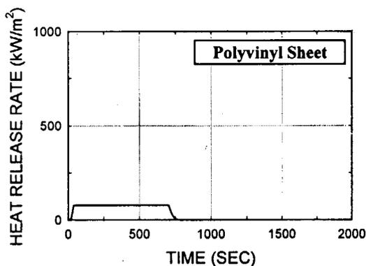
Fig. D23. Polyvinyl chloride, 0.5 in thick (test 333), Sheet
