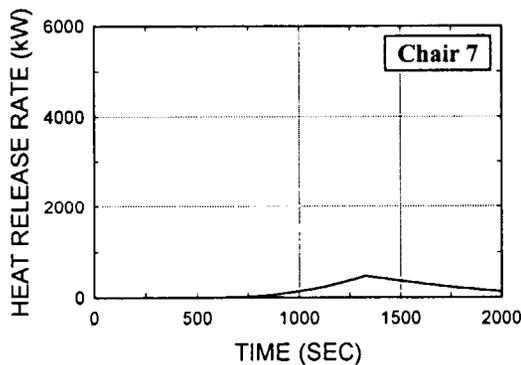
Fig. B9. Chair, molded flexible pu frame, pu cover test 64 (83-2787)
