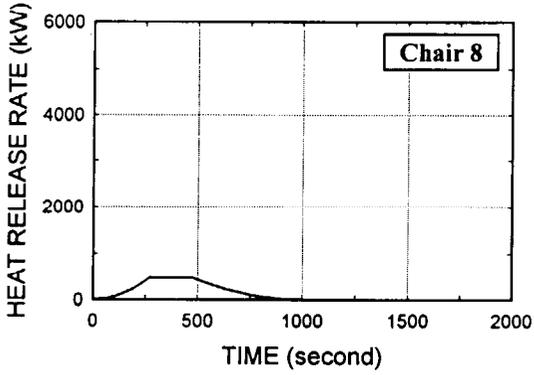
Fig. A13. Chair, wood frame, FR cotton stuffing, polyolefin fabric
