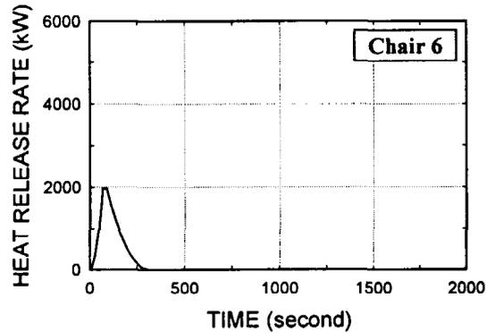
Fig. A11. Chair, wood frame, California foam, polyolefin fabric
