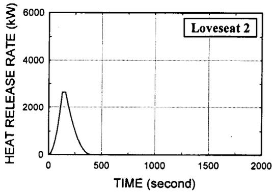
Fig. A25. Loveseat, wood frame, California foam, polyolefin fabric
