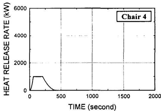
Fig. A9. Chair, urethane foam frame, urethane foam, polyolefin fabric
