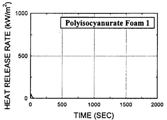
Fig. D17. Rigid polyisocyanurate foam, 2 in (test 438), Foam
