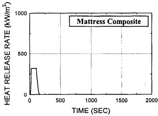
Fig. D7. Mattress ass'y m05, pu foam, rayon ticking (test 296), Composite
