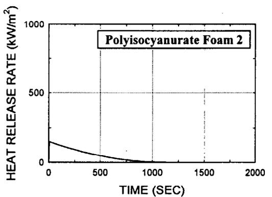
Fig. D18. Rigid polyisocyanurate foam, 2 in (test 449), Foam
