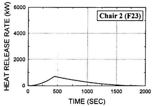
Fig. B4. Chair, F23, wood frame, fr cotton batting, olefin test 24(82-2604)
