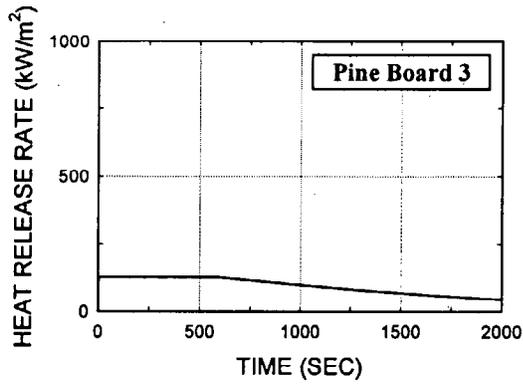
Fig. D13. White pine (wood), 0.75 in (test 487), Board
