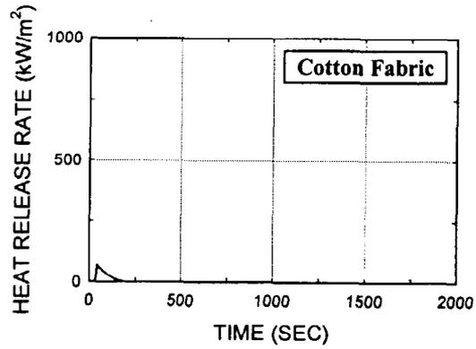
Fig. D1. Cotton fabric, fr (test 803a), Fabric
