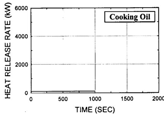
Fig. B12. Cooking Oil, Corn; Cottonseed; Etc In 12in.Pan
