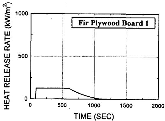
Fig. D3. Douglas fir plywood, 1/2 in. thick (435), Board
