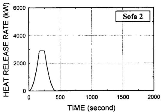
Fig. A31. Sofa, wood frame, California foam, polyolefin fabric
