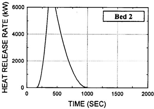
Fig. B2. Double bed, bedding, night table; plywood walls; test R5 (85-2998)
