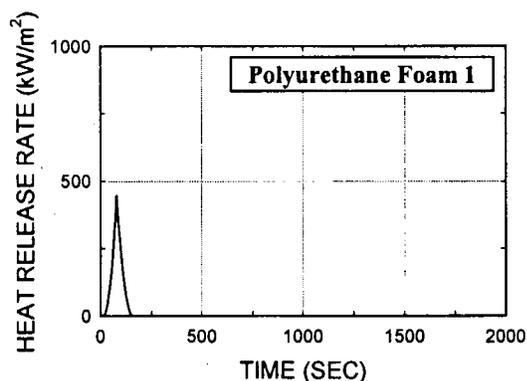
Fig. D20. Flexible polyurethane foam, fr, 2 in (test 725), Foam
