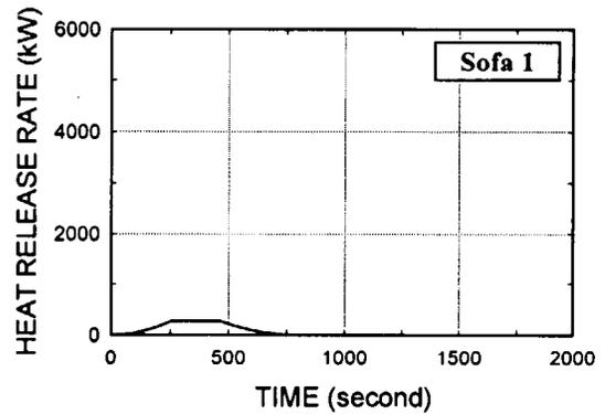
Fig. A30. Sofa, metal frame, urethane foam, plastic-coated fabric
