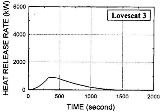
Fig. A26. Loveseat, wood frame, urethane foam, plastic-coated fabric
