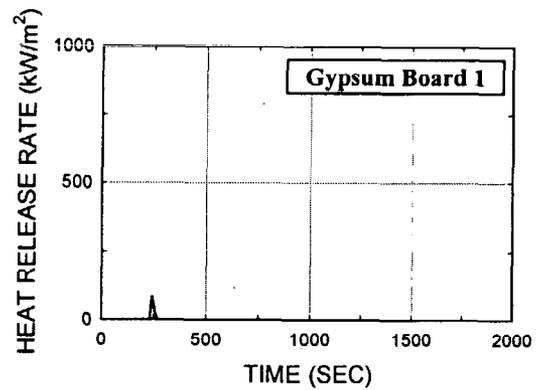
Fig. D5. Gypsum board, 1/2 in. thick (434)
