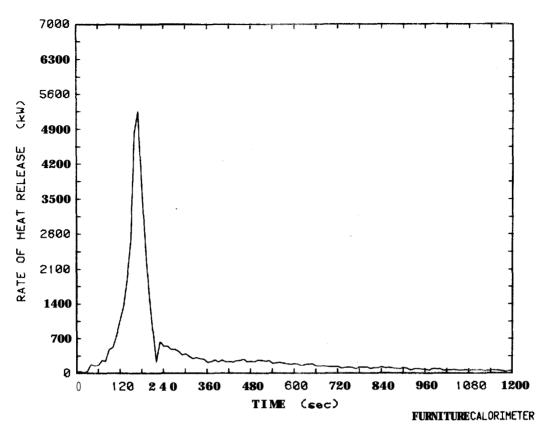
Figure 108. Rate of heat release plot for 3.2 mm plywood wardrobe painted inside with one coat if fire-retardant paint, Test 42
