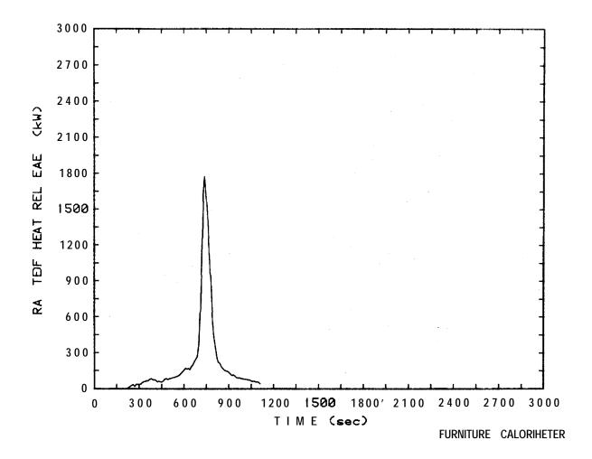
Figure 82. Rate of heat release plot for mattress Test 74
