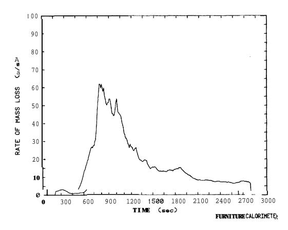
Figure 75. Rate of mass loss plot for wood frame loveseat, Test 57
