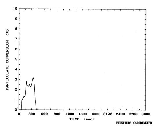
Figure 67. Smoke particulate conversion plot for sofa with "California foam" cushions, Test 38
