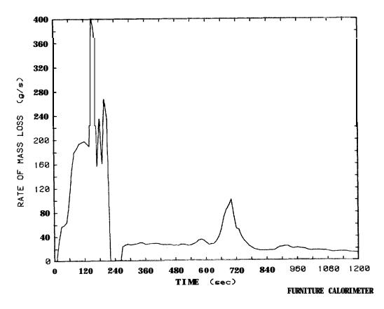
Figure 92. Rate of mass loss plot for 12.7 mm plywood wardrobe, Test 39
