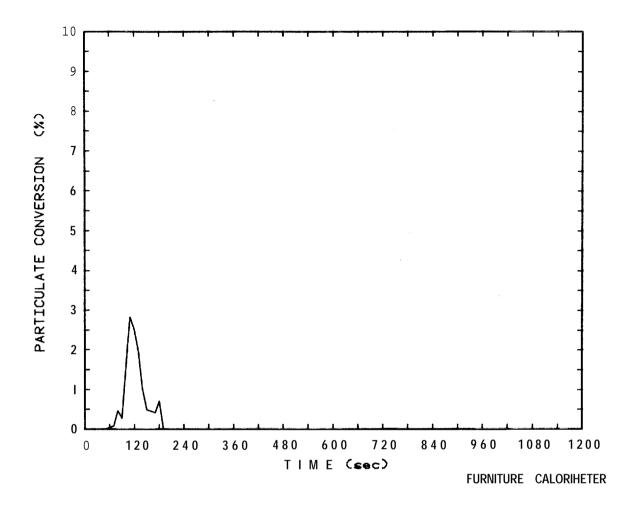
Figure 112. Smoke particulate conversion plot for 3.2 mm plywood wardrobe painted inside with one coat of fire-retardant paint, Test 42
