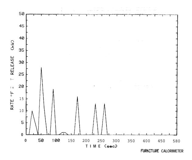
Figure 126. Rate of heat release plot for 12.7 mm wood bookcase, Test 62
