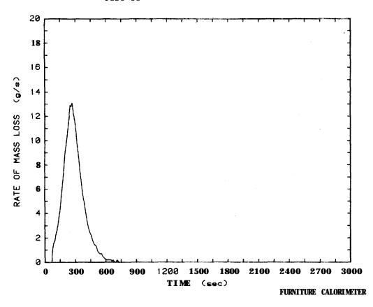
Figure 45: Rate of mass loss plot for metal frame chair, Test 53
