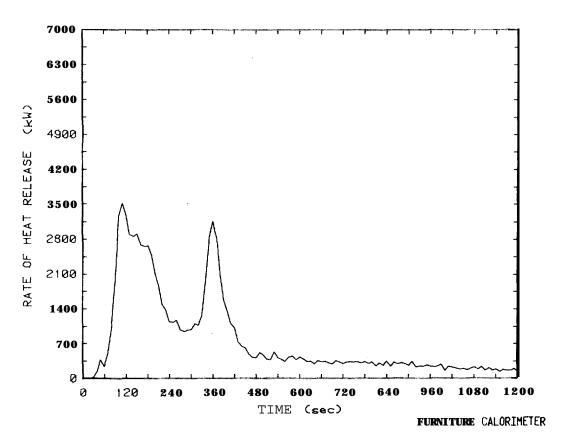
Figure 95. Rate of heat release plot for 12.7 mm plywood wardrobe, Test  $\mathbf{40}$
