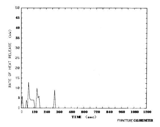
Figure 49: Rate of heat release plot for chair from group setting, Test 55
