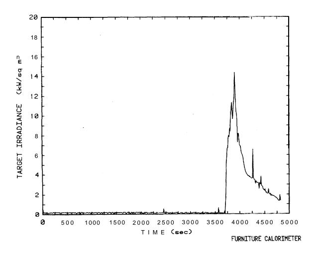
Figure 25. Target irradiance plot for easy chair Test 66
