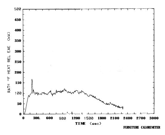
Figure 59: Rate of heat release plot for metal frame stackable chairs, Test 75
