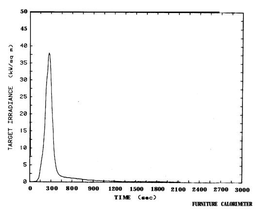
Figure 66. Target irradiance plot for sofa with "California foam" cushion, Test 38
