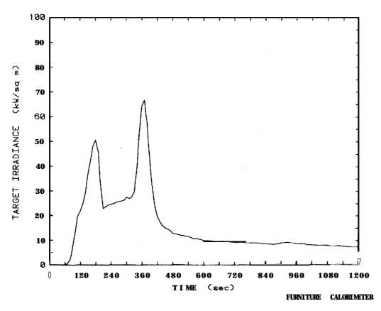
Figure 101. Target irradiance plot for 12.7 mm plywood wardrobe, Test 43
