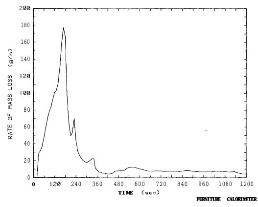
Figure 114. Rate of mass loss plot for 3.2 mm plywood wardrobe painted inside and out with two coats of fire-retardant  ${\bf 1}$ atex paint Test 44
