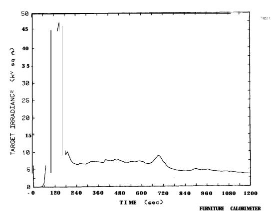
Figure 93. Target irradiance plot for 12.7 mm plywood plywood wardrobe Test 39
