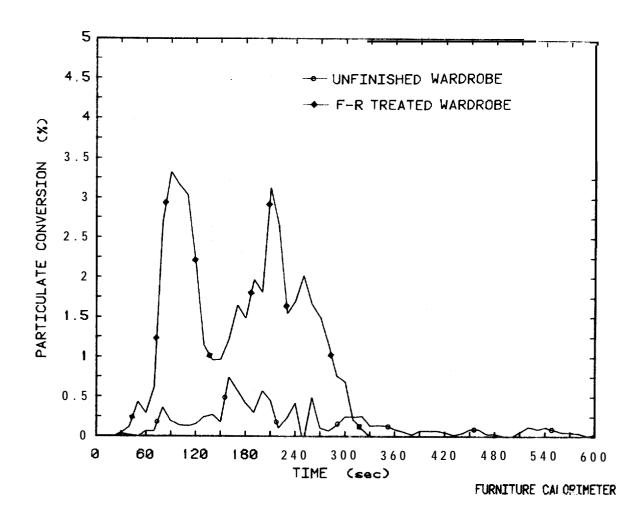
Figure 119. Comparison of smoke particulate conversion for Tests 41 and 44
