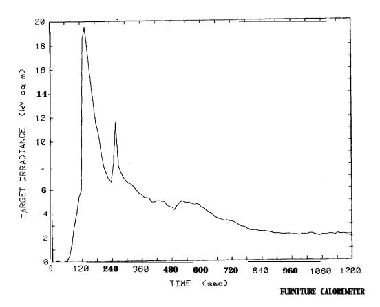
Figure 106. Target irradiance plot: for  $3.2\ \text{mm}$  plywood wardrobe, Test 41
