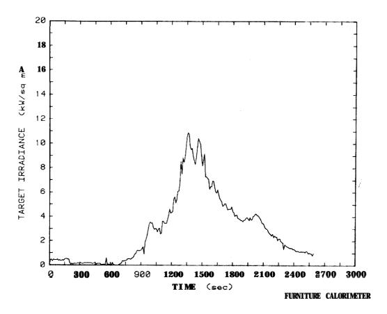
Figure 20. Target irradiance plot for easy chair Test 64
