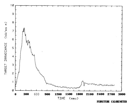
Figure 15. Target irradiance plot for easy chair Test 49
