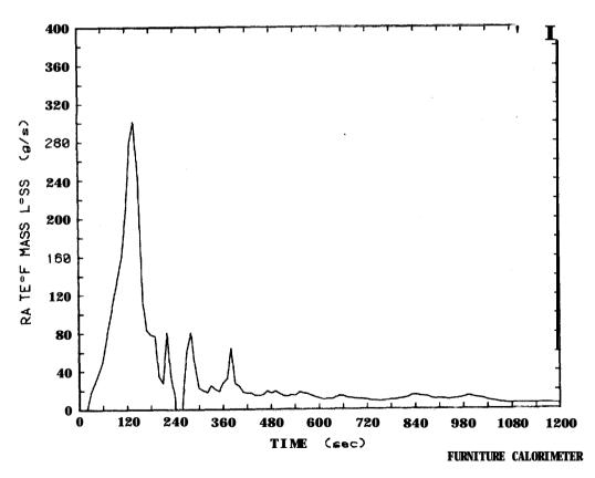
Rate of mass loss plot for 3.2 mm plywood wardrobe, Figure 105. Test 41
