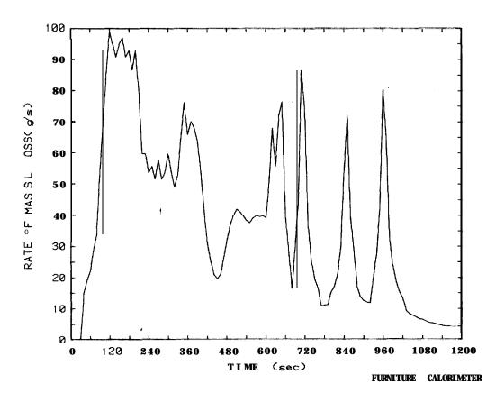
Figure 96. Rate of mass loss plot for 12.7 mm plywood wardrobe, Test  $40\,$
