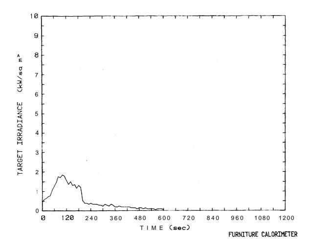
Figure 37. Target irradiance plot for molded fiberglass chair Test 51
