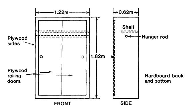
Figure .03. Photograph and sketch of 3.2~mm plywood wardrobe
