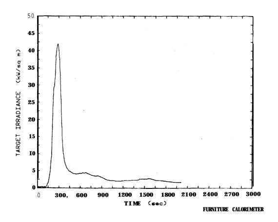
Figure 5: Target irradiance plot for easy chair, Test 45
