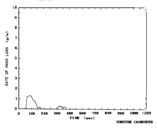
Figure 36: Rate of  ${\bf mss\ loss}$  plot for molded fiberglass chair, Test 51
