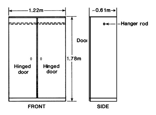
Figure 90. Photograph and sketch of 12.7 mm plywood wardrobe
