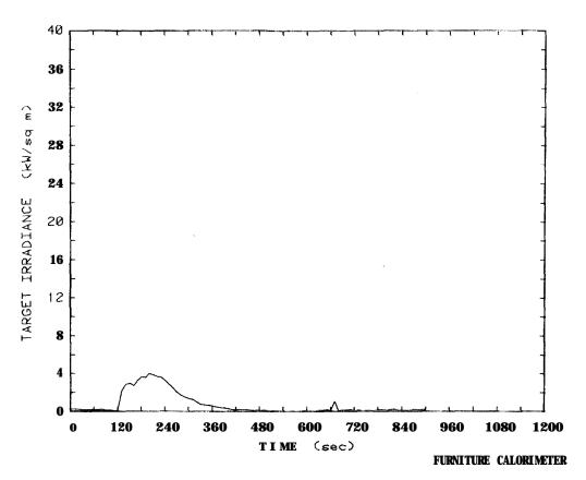
Figure 88. Target irradiance plot for metal wardrobe, Test 21
