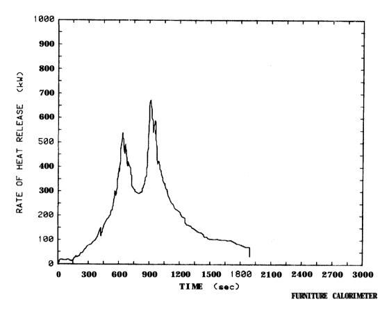
Figure 79. Rate of heat release plot for mattress and boxspring, Test 67
