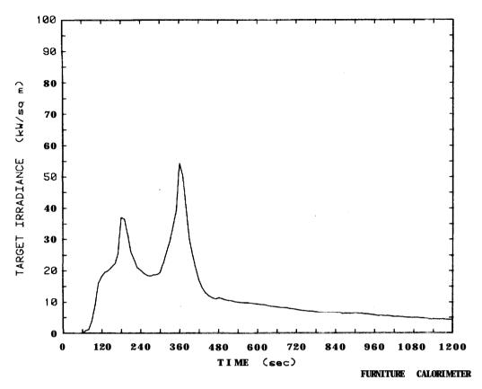
Figure 97. Target irradiance plot for 12.7 mm plywood wardrobe, Test 40
