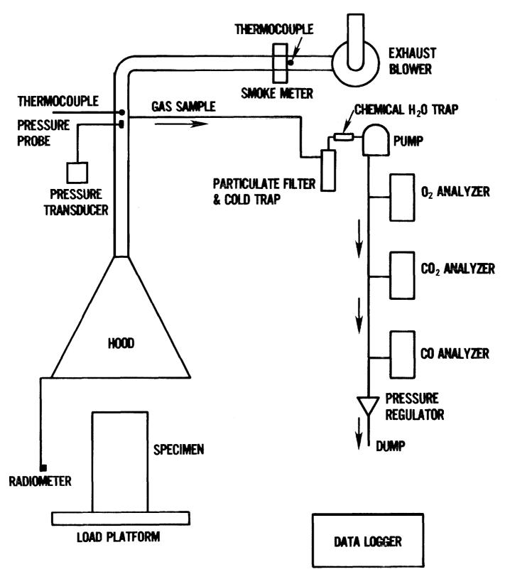
Figure 1. Furn ture calorimeter, schematic of flow and instrumentation
