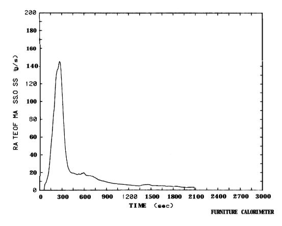
Figure 65. Rate of mass loss plot for sofa with "California foam" cushions, Test 38
