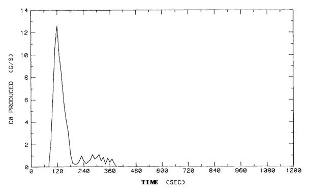
Figure 111. Carbon monoxide production plot for 3.2 plywood wardrobe painted inside with one coat of fire-retardant paint, Test 42
